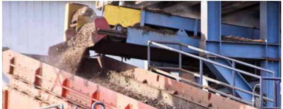
The shredder can process 4,000 tons of scrap in a 40-hour work week.
